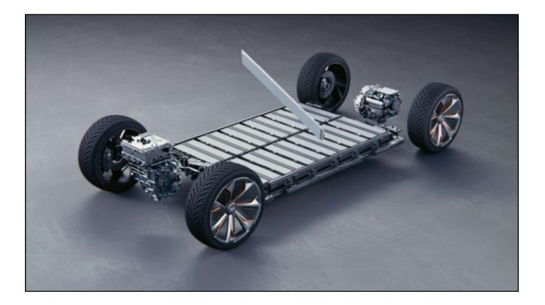
GM's transition into an all-electric future revolves around its new Ultium Battery System, which is shown here.
